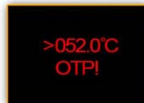
Over temperature alarm
